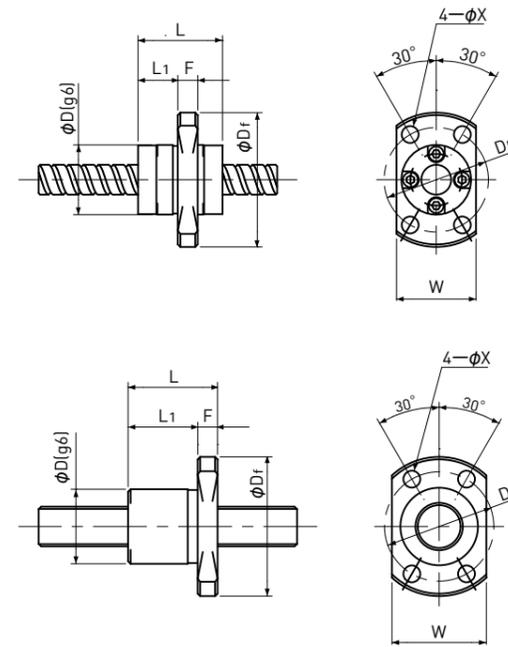
Type-2 : End-cap type (Ball Screw Nut)
