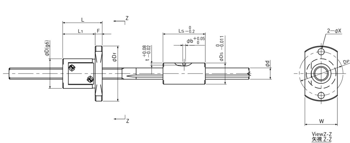
Type-1 : Return-plate type (Ball Screw Nut)
