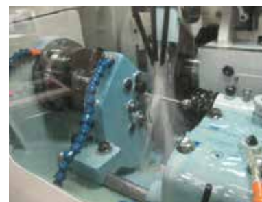
ねじ研削盤による高精度ねじ溝加工 High accurate shaft groove process by Grinding machine
